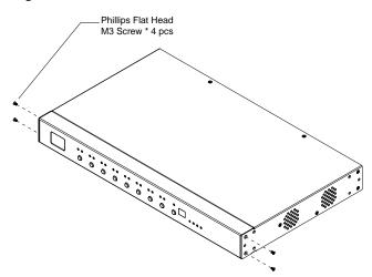
2. Use the screws you just removed, and the ones supplied with the rack mounting kit to screw the rack mounting brackets into both modules:
