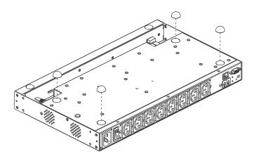
**Note:** To ensure adequate ventilation, allow at least 5.1 cm on each side, and 12.7cm at the back for power cord and cable clearance.
